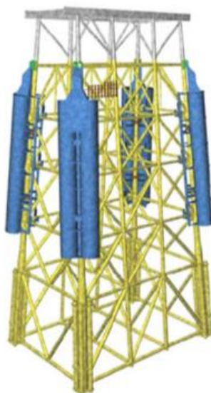
Figure 6 Scheme of the buoyancy tanks attached to the four corner legs to remove Frigg structure (Frigg Field Cessation Plan, 2011).
