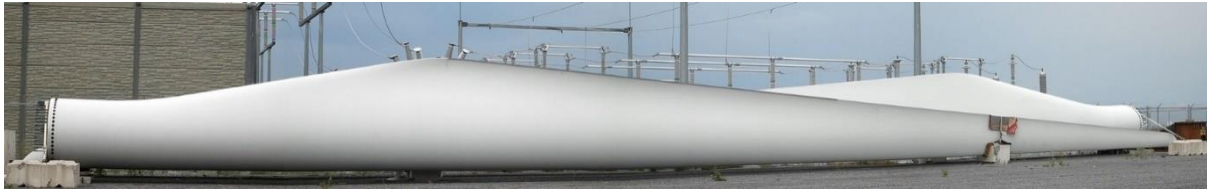
Figure 3: Fiberglass-reinforced epoxy blades of Siemens SWT-2.3-101 wind turbines. The blade size of 49 meters[43] is in comparison to a substation behind them at Wolfe Island Wind Farm. 1
