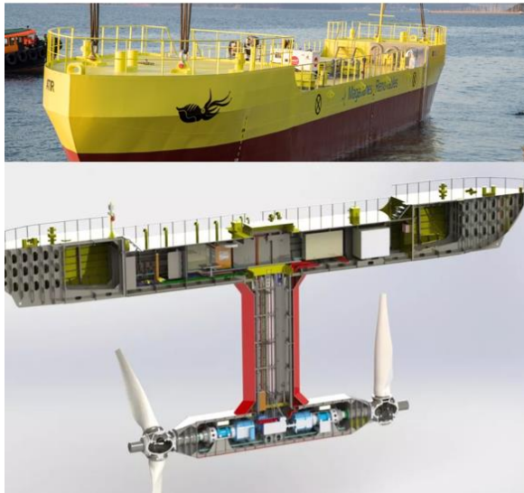
Figure 8: Examples of floating tidal turbines.
