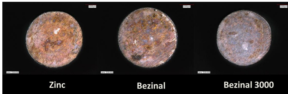
Figure 12: Pictures of cut edges of 4 mm steel wires with Zinc, Benzinal and Benzinal 3000 coatings after 3 years of exposure in Belgium [111]
