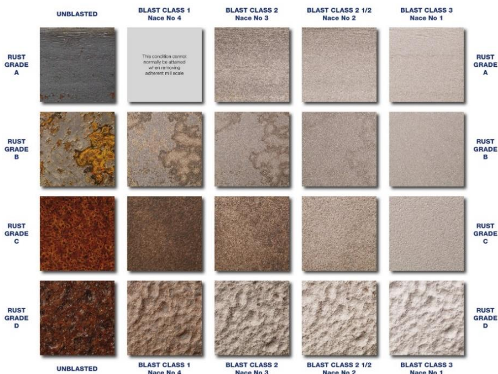
Figure 10: Surface aspects of cleaned surfaces in function of the rust grade according to ISO 8501-1
