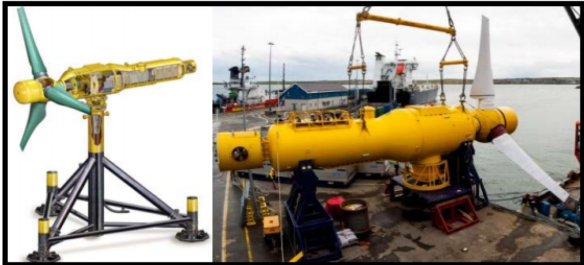
Figure 20 – ALSTOM tidal turbine DEEP-Gen IV EMEC testing programme for ReDAPT [43]
